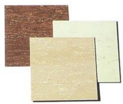
Top quality smooth surface rubber floor tile. Colors match stair covering materials; extend throughout thickness for long wear. Offers the durable, resilient, long- wearing, easy maintenance of rubber flooring. Contains no asbestos fiber. Meets Fed. Spec. SS-T-312B. Install with Musson #560 Rubber Flooring or #775 Epoxy Adhesive.
