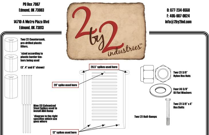
This ADA Ramp has been designed to work universally with any manufacturer's plastic border timber, provided its method of attachment involves a 3/4" diameter steel spike. You have the freedom to use 6", 8", or 12" plastic playground border timbers because the attachment point sits BENEATH the timber.
