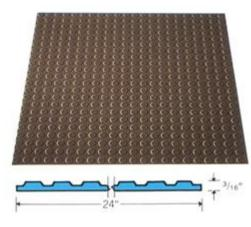
This unique floor tile with raised circular discs (3/4" diameter), for better traction; is attractive, non-staining and non-discoloring. Factory cut 24" x 24" square tiles mean quick installation, fewer joints. Circular discs allow for easy cleaning. Wheeled equipment moves across easily. Ideal for stair landings, lobbies, entrances, elevators, hallways, ramps; around concessions or vending machines.
