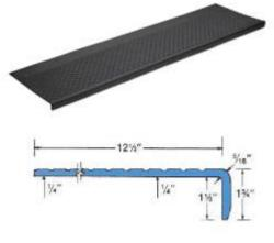
Our new No. 633 Outdoor Rubber Stair Tread is an excellent stair tread for exterior applications. This tread, made from 100% recycled tires, is available in black color only in a diamond pattern with a 3" smooth back border in square nose pattern only.
