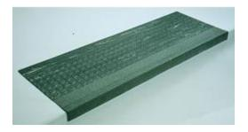
Available with 2" wide, long wearing mineral coated Grit Strips recessed the full length of the tread at impact area. Helps prevent slipping. Design surface with Grit Strips offer added safety and longer wear. All treads have color through entire thickness. All treads meet Flame Spread Rating of 75 or less using ASTM-E-84 Test.
