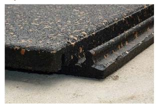
This patent pending interlocking edge design works in a way that is reminiscent of that used in some common resealable plastic bags. On each edge of the PopLock tiles, there is an oval-shaped male ridge or a similarly shaped female groove. When these components are pressed together, a strong, shift resistant edge connection is created. These tiles can be joined together or separated in seconds, over and over again.
