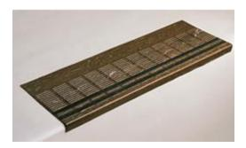
Available with two 3/4" wide, long wearing mineral coated Grit Strips recessed the full length of the tread at impact area. Helps prevent slipping. Design surface with Grit Strips offer added safety and longer wear. All treads have color through entire thickness. All treads meet Flame Spread Rating of 75 or less using ASTM-E-84 Test.
