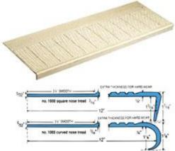
An attractive, easy to clean, horizontal bar pattern, with a tapered return nose for better fit. Extra thick front edge tapers to smooth rear border, makes cleaning easier. Meets Federal Specs. RR-T-650E and ZZ-T-001237 (GSA-FSS). Install with Musson No. 400 Neoprene Contact, No. 300 Water-base Contact Adhesive or No. 560 Rubber Flooring adhesive.
