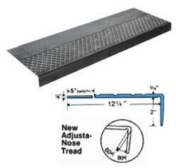
A New Design Nose - will easily adjust and adhere to steps with return angle nosings between  $90^{\circ}$  and  $60^{\circ}$ ; allows good fit on stairways designed for safety or aesthetics.
