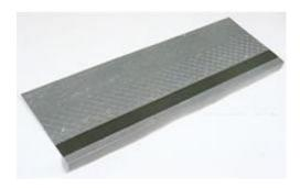
Available with one 2 " wide, long wearing mineral coated Grit Strips recessed the full length of the tread at impact area. Helps prevent slipping. Design surface with Grit Strips offer added safety and longer wear. All treads have color through entire thickness. All treads meet Flame Spread Rating of 75 or less using ASTM-E-84 Test.
