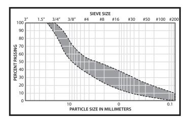
The above sieve analysis is the ideal curve for a simple and long lasting packed aggregate sub-surface. Since a packed aggregate base is subject to potential movement, we recommend staying within the above gradient to reduce sub-surface movement possibility.
