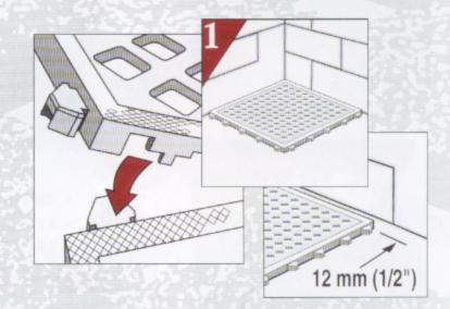
Where the edge of the mats are exposed to any traffic, safety ramps should be fitted using the simple push to lock method.
