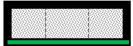
**OVERVIEW:** For best overall function and appearance, fasten the first screw exactly halfway up the strip, close to the far edge of the strip. Next, fasten the top row of screws approximately 12" apart, followed by the bottom row of screws approximately 12" apart, staggered with the top row. Finish the strip by fastening the final screw exactly halfway up the strip, close to the far edge.
